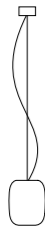
S1 Ceiling Rose Ø 80 mm Ceiling Rose LED Ø 160 mm Cable 2000 mm Diffuser Ø 180 mm H 210 mm
