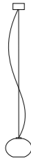
S1 Ceiling Rose Ø 80 mm Cable 2000 mm Diffuser Ø 175 mm H 120 mm
